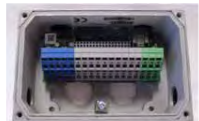
Example: external BUS adapter unit SK TI4-TU-BUS
